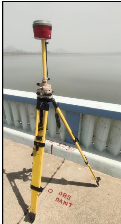
Figure 5.3-1 RTK BASE SET UP
